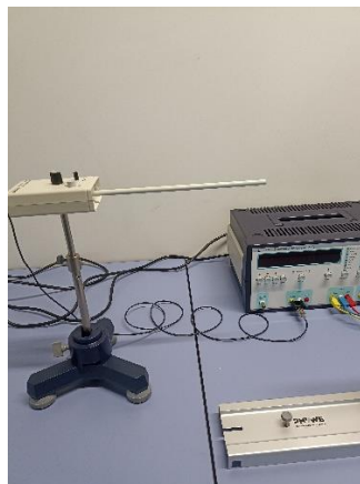
Fig. 3. Connecting the microphone to the universal counter
